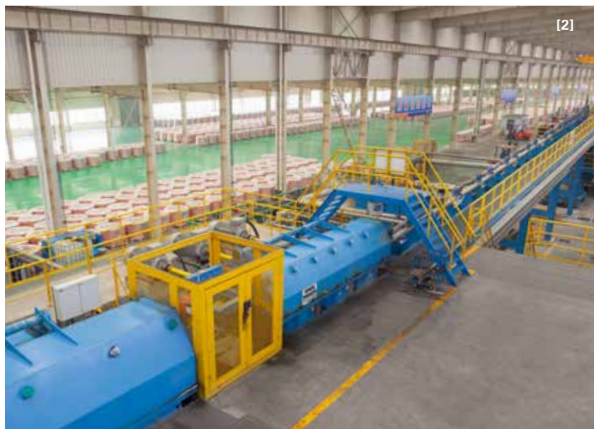
[1] | Modern technology cuts energy consumption. [2] | The copper wire is rolled in a closed system.
